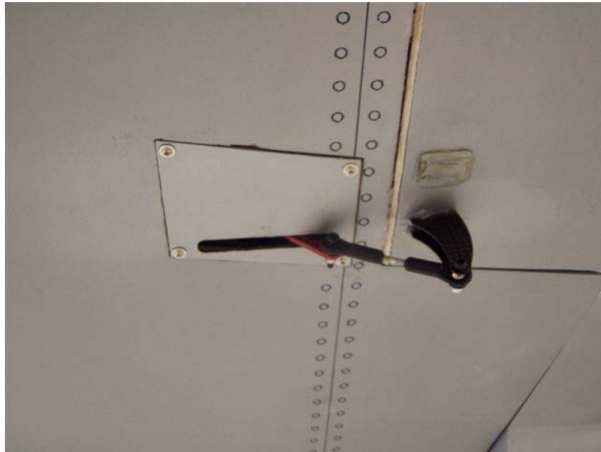
This photo shows the position of the flap horn. It is in the up position here.
