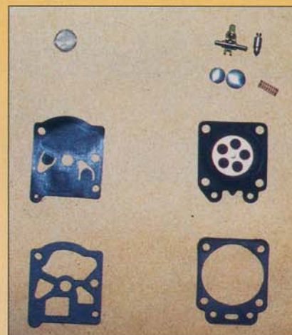
This photo depicts the carb rebuild kit. Notice the two bowl shaped Welsh plugs and the large washer on the metering diaphragm.
